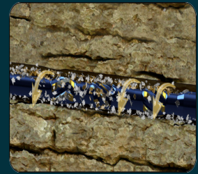
Cuttings and fluid move uniformly in annulus with CBM's in the drill string.
